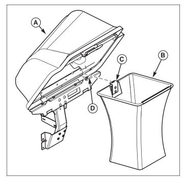
Figure 7. Install Collector Bags A. Cover
